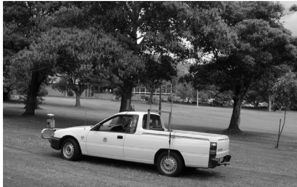
Figure 12.12 The vehicle used in our experiments is equipped with a 2D laser range finder and a differential GPS system. The vehicle’s ego-motion is measured by a linear variable differential transformer sensor for the steering, and a wheel-mounted velocity encoder. In the background, the Victoria Park test environment can be seen.
