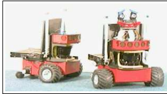
Figure 14.5 RWI Pioneer robots used for multi-robot mapping. These robots are equipped with a SICK laser range finder.
